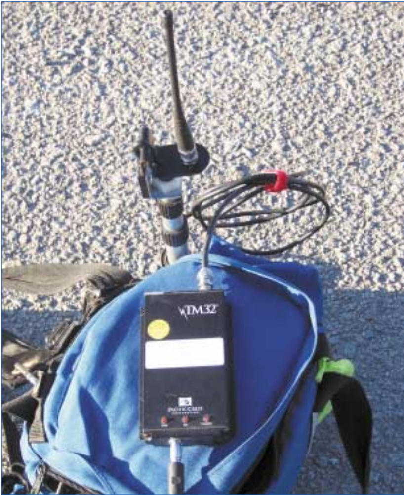
Fig 2 – TM32 2 watt rover radio - note data & power feed (from GPS receiver) and extension cable for small whip antenna.
