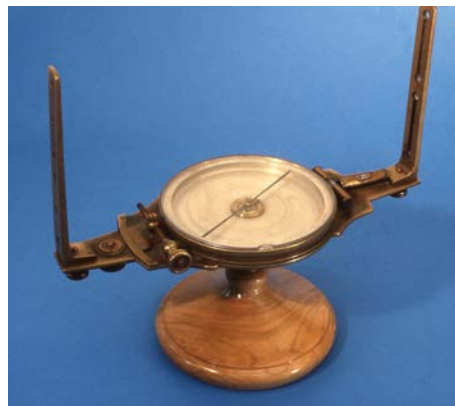
The standard American vernier compass by W. & L.E. Gurley. This form with vernier, outkeeper, sights, level vials, was made from about 1860 and remained in the Gurley catalogs into the 1930s. It attached to either a tripod or Jacobs Staff.
