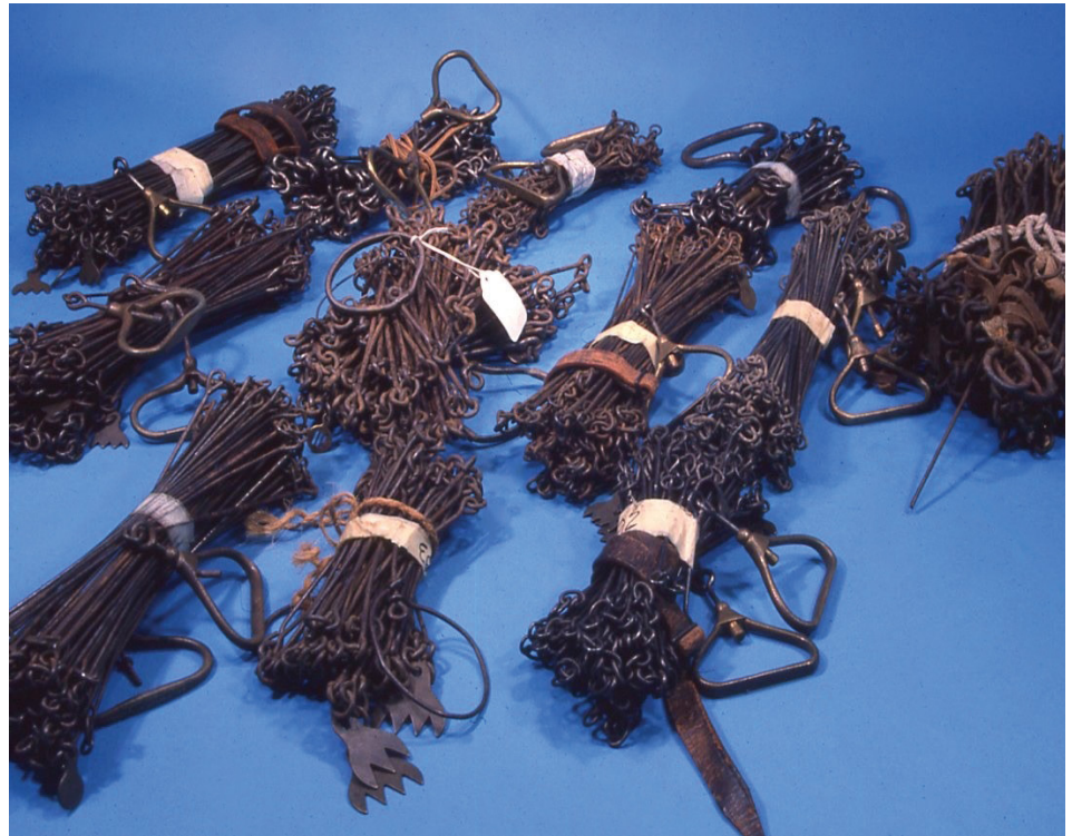
An assortment of chains: Gunter's Chain, 66 feet. A half-chain, 33 feet. Railroad or Engineer's Chain, 100 feet.
