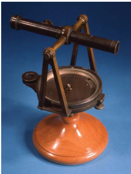
This is one of the first transits made in America. William J. Young, Philadelphia. Three minute least count, bullseye bubble. Was made in the very early 1830s.
