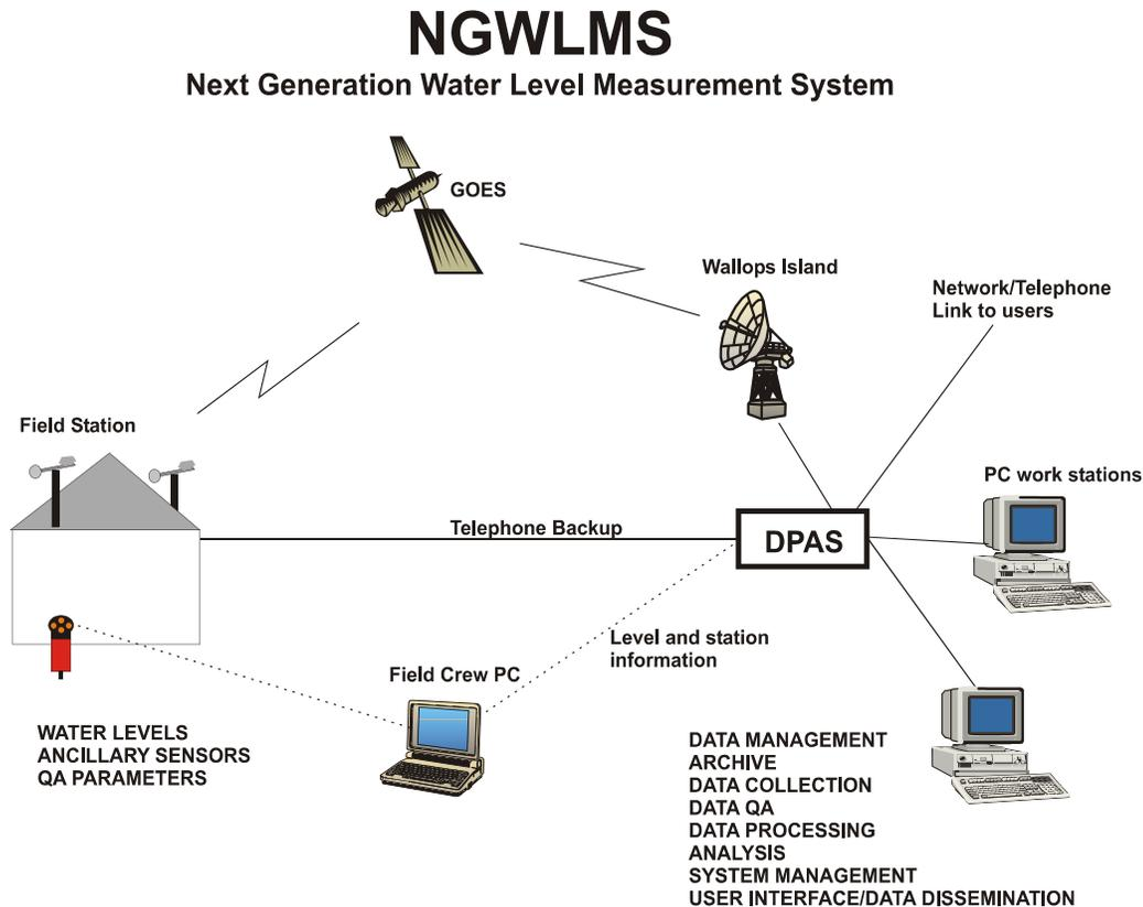
**Figure 15.** A schematic diagram of the main systems associated with NGWLMS.
