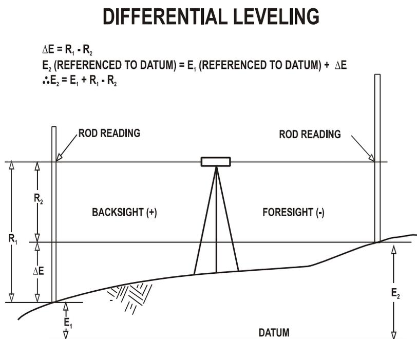
**Figure 13.** A schematic diagram of extending vertical control inland from the tidal datum by the method of differential leveling.
